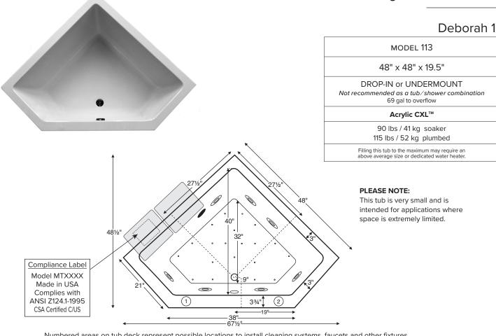
Numbered areas on tub deck represent possible locations to install cleaning systems, faucets and other fixtures. Pump extends 6" beyond edge of tub.
