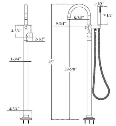
Use on concrete floors requires special installation. We recommend using a plumbing proffessional. Dimensions are nominal and may vary. Dimensions and specifications subject to change without notice.
