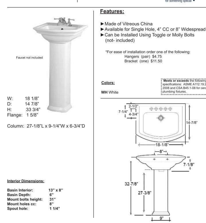
Dimensions of fixture are nominal and may vary within the range of tolerances established by ASMEI Standard A112.19.2-2008. Dimensions and specifications subject to change without notice.
