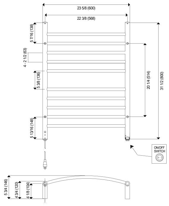
Note: Drawing shows back of unit. Power connection on the right when mounted on wall.
